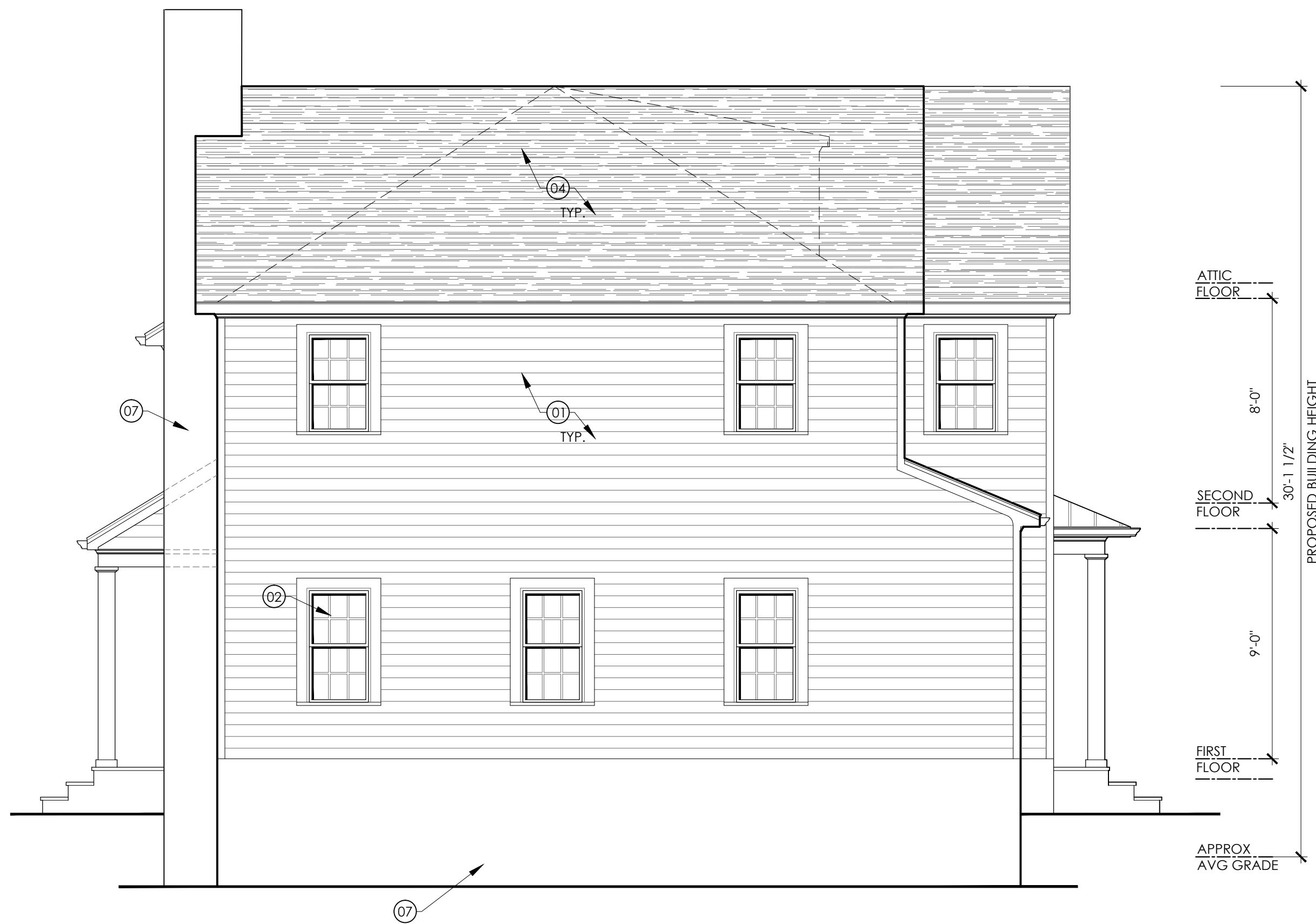
02 PROPOSED LEFT SIDE ELEVATION SCALE: 1/4" = 1'-0"
