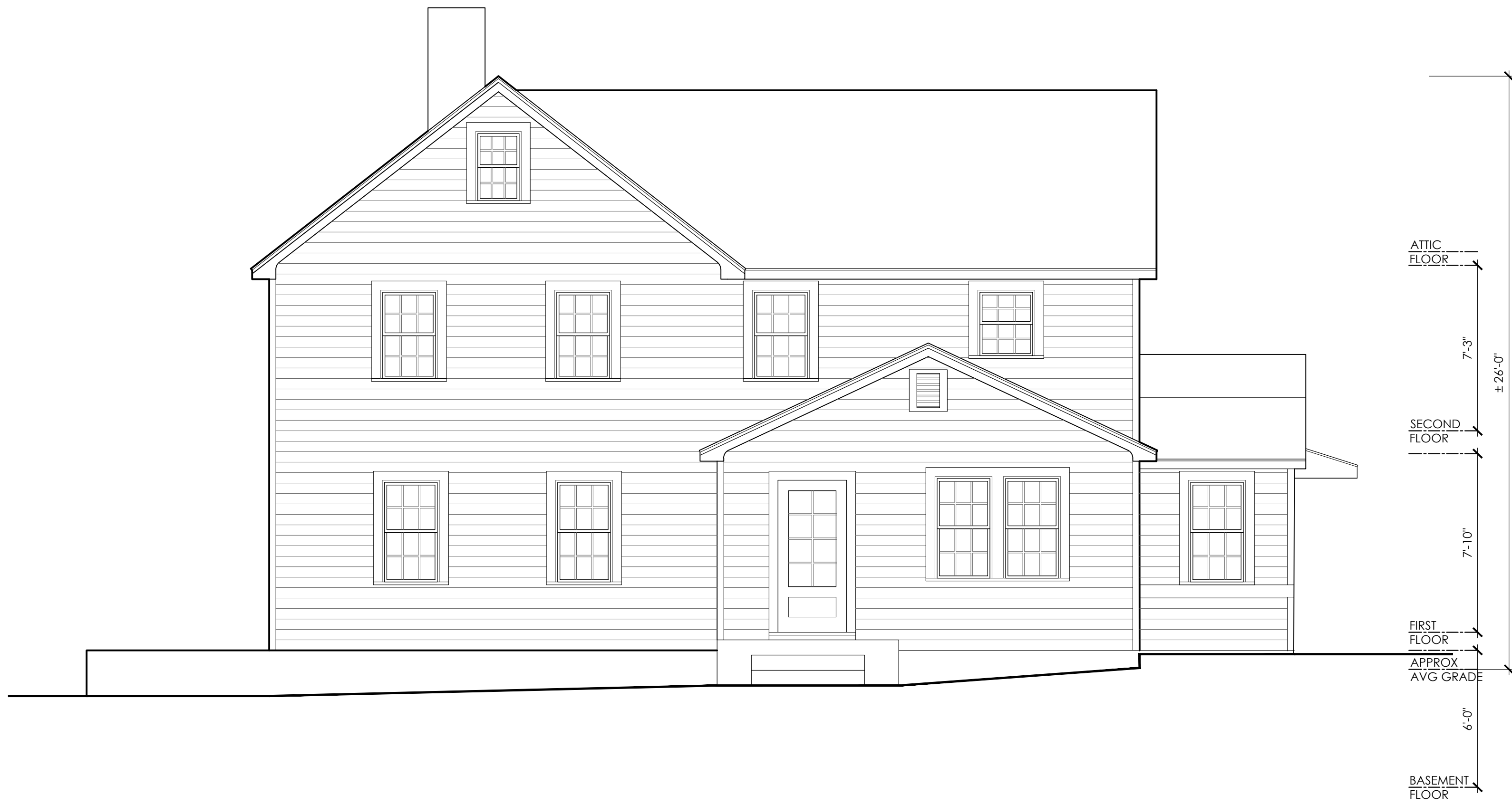
01 EXISTING FRONT ELEVATION SCALE: 1/4" = 1'-0"
