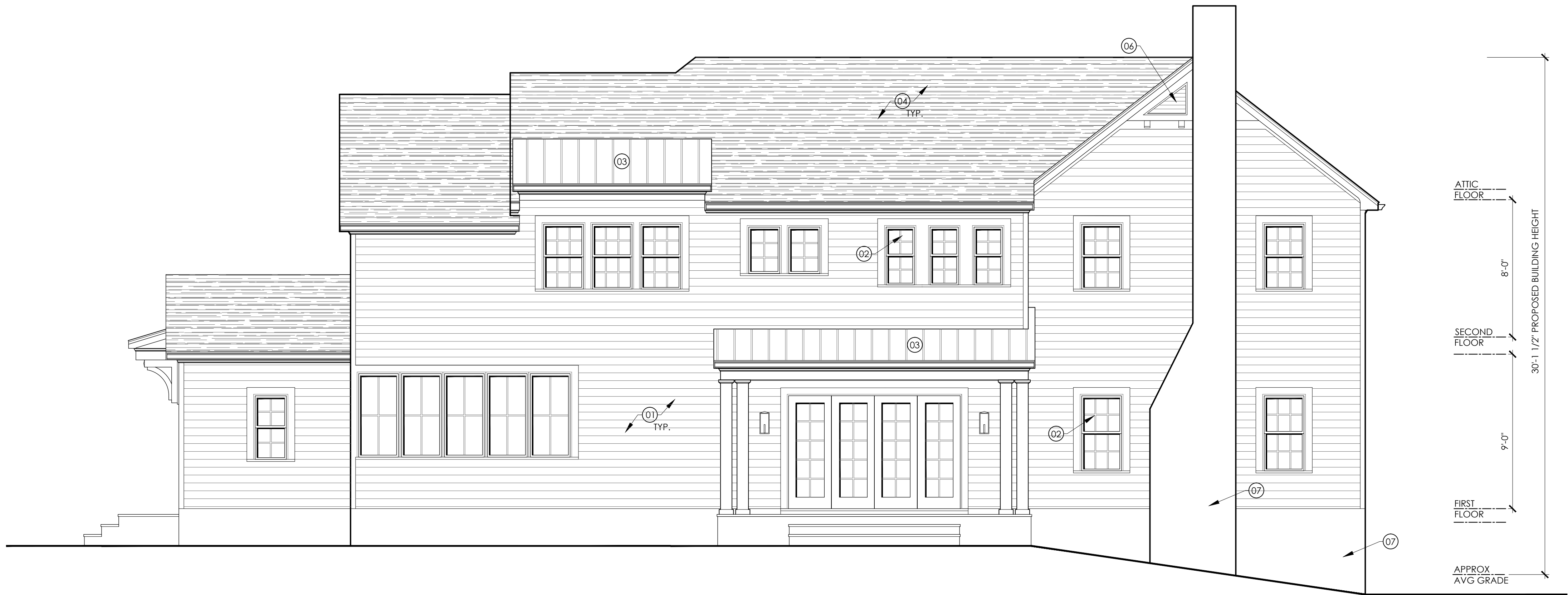
01 PROPOSED REAR ELEVATION SCALE: 1/4" = 1'-0"
