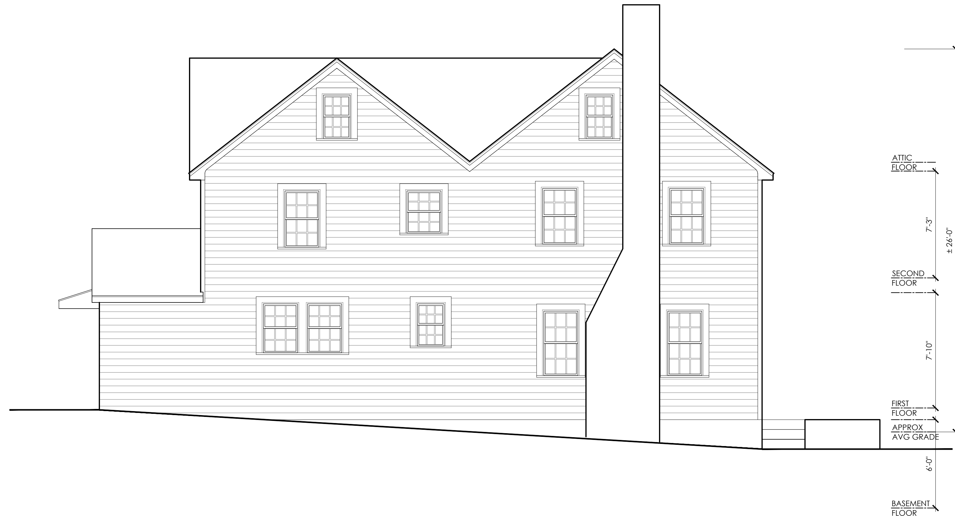
03 EXISTING REAR ELEVATION SCALE: 1/4" = 1'-0"
